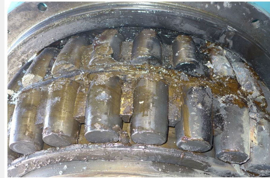
Fig 1: Main bearing failure due to bearing wear. (windpowerengineering.com)
