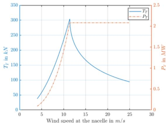
Figure: Thrust force and electric power of a 78 m rotor wind turbine.
