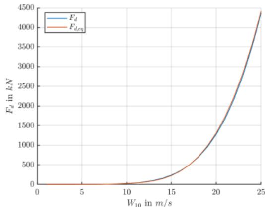
Figure: Mean wave drift force.
