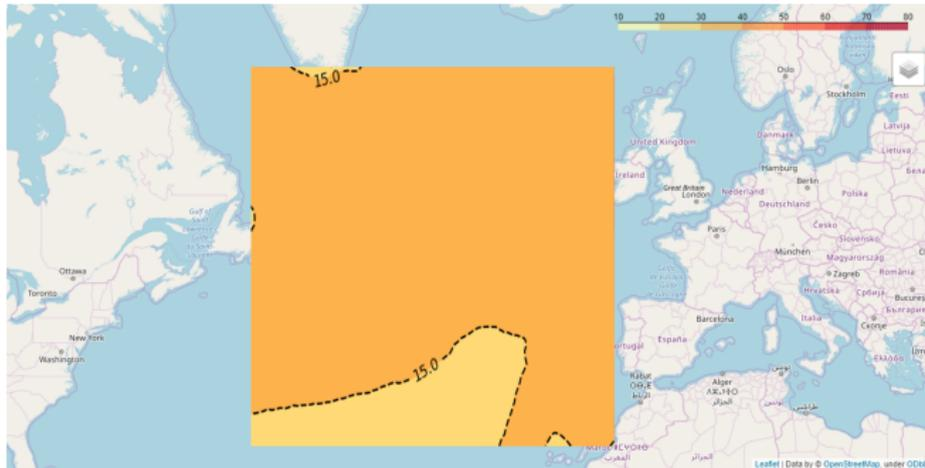
**Figure:** Mean CF of a dynamically positioned wind turbine deployed in the North Atlantic ocean - From 2015 to 2017.
