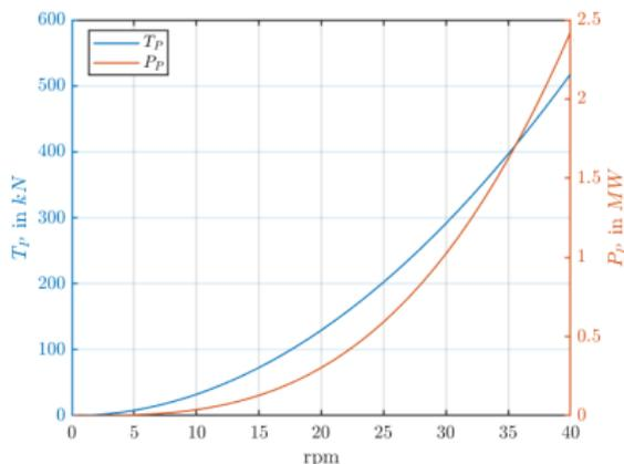
Figure: Propellers thrust force and consumed power for an inflow velocity of 0 m/s.
