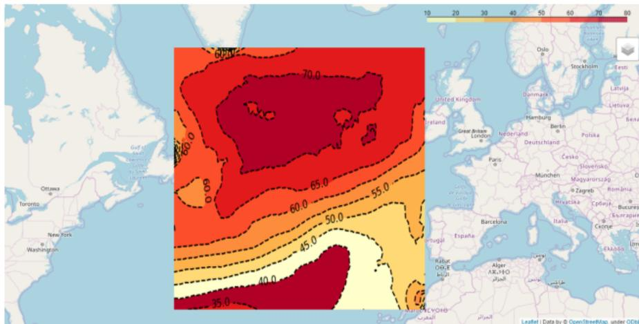
**Figure:** Mean CF of a stationary wind turbine deployed in the North Atlantic ocean - From 2015 to 2017.
