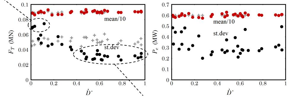
Note that the standard deviation of thrust is limited to the low-frequency component, and, as seen in the plot, it does not directly correspond to the component damage metric. These turbines, experiencing high levels of turbulent loading, are rejecting part of the low-frequency thrust fluctuations
