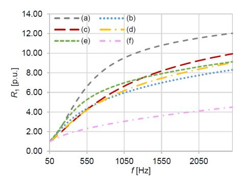
Submarine cable equivalent frequency-dependent positive-sequence resistance assuming:
