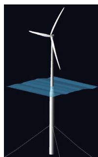
Figure 6. Model of FOWT in FAST code
