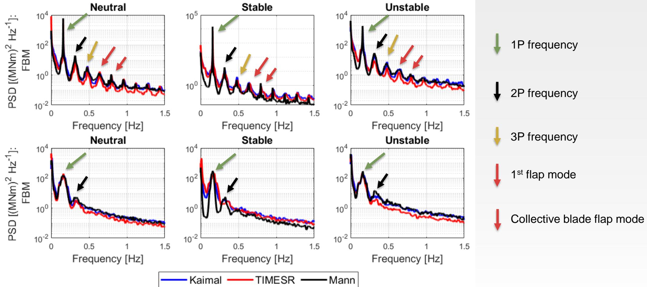
Close to rated wind speed ( $\pm 12.5 \text{ m/s}$ )
