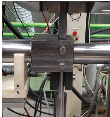
Figure 2. Friction test set-up with specimens tested in air.
