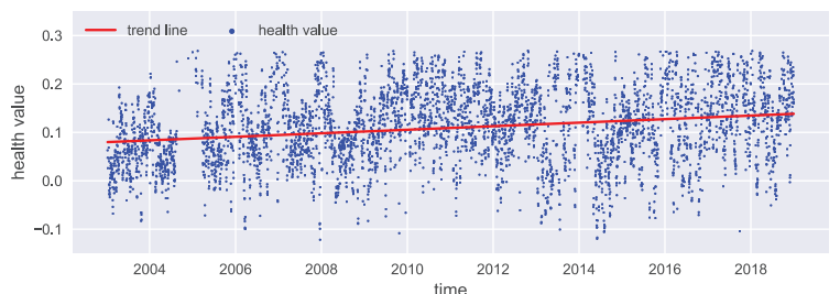
Figure 4: Long term power curve degradation of a German onshore wind turbine over 16 operational years. A linear regression highlights a trend in daily health values. Health values above the normal process control limit were deleted from the data set to exclude temporary technical issues.
