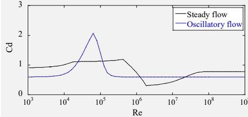
Figure 2  $C_d$  of a circular cylinder in the steady and oscillatory flows
