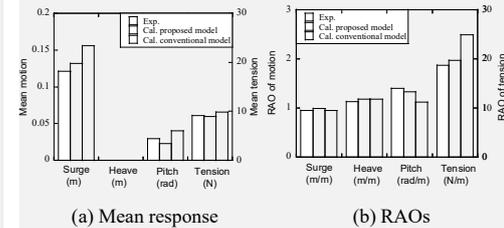
Figure 4 Comparison of predicted responses by the proposed and conventional models in the wave and current case (H=0.06m, T=2.5s, v=0.2m/s)
