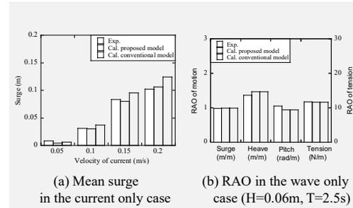
Figure 3 Comparison of predicted responses by the proposed and conventional models in the wave-only and current-only cases
