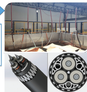
Manufactured, pretested, preconditioned, 2 years ageing test of FLOTANT XLPE insulated 66kV submarine cable core (FULGOR facilities, Greece)
