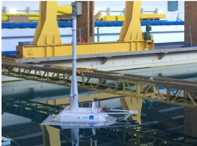
Characterization tests: decay; tilt; pull out
