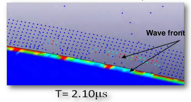
first impact, shockwave After the а propagate inside the particle field, disturbing it, spoiling the results.
