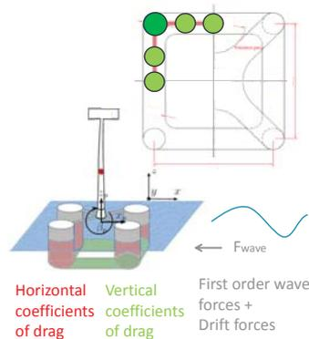
Fig 2: hydrodynamic drag and wave forcing on model
