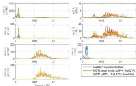
Fig 4: PM Extreme irregular wave spectrum test comparison
