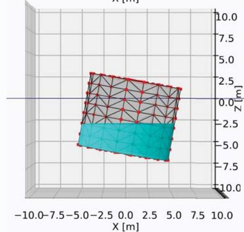
Due to the cylinder geometry, the effect of the liquid ballasting produces a considerable increasing of the pitch period of the structure. Also an amplitude increment of the related frequency is noted considering liquid ballasting instead of granular ballasting (about 8%).
