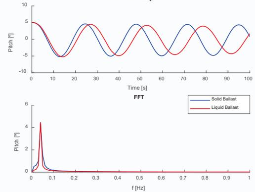
In this case, the influence of the ballast model is less accused than in the cylinder due to the geometry of the platform, but as shown in time domain analysis, the period of the platform is slightly shifted and also the amplitude associated increases about 4% with liquid ballasting.
