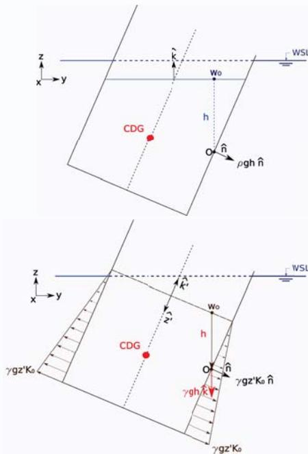
Granular ballast model is reduced to rotations smaller than the internal friction angle, to ensure that free surface remains parallel to the base. For liquid ballast, only a vertical hydrostatic distribution is applied, thus the structure needs quasi-static movements with low inertial accelerations and also with a frequency movements far enough from sloshing phenomena, which is no modeled in this approach.
