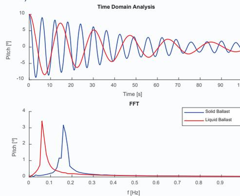
Second simulation is based on a FEM model of the DeepCwind semisubmersible platform, composed of 48 beam and 2592 shell elements. The initial pitch rotation is fixed in 5 degrees from the equilibrium position.
