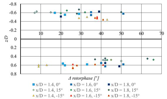
Figure 3: Vortex core sizes in degrees for three downstream positions, left and right side of the wake.
