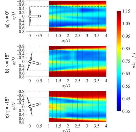
Figure 2: Interpolated normalized streamwise velocity. a) non-yaw reference case, b) positive yaw angle, c) negative yaw angle
