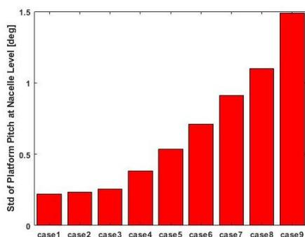
Figure 1. Sensitivity of changing  $H_s$  and  $T_p$  in below the rated wind speed (wave characteristics vary from case 1 where  $H_s=0.75$ m and  $T_p=6.5$ s to case 9 where  $H_s=12.25$ m and  $T_p=15.5$ s)
