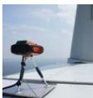
Nacelle mounted Lidar delivers accurate measurements, across multiple turbines, at a significantly lower cost point, with high availability and low uncertainties.
