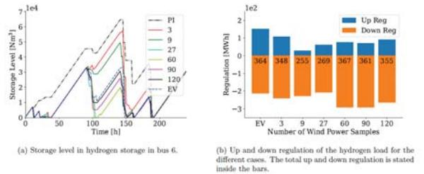
Figure 5: Hydrogen storage level and regulation of the hydrogen plant.
