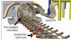
Forms are equipped with 4 sets of wheels matching rails on reception lane.
