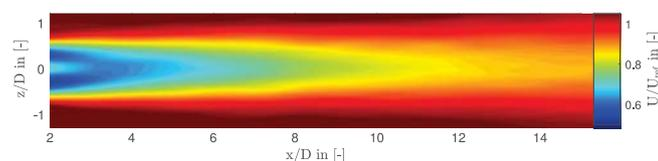
Figure 2: Wake measurement result at  $I_a = 10\%$  and  $\beta = 0^\circ$  from  $x/D = 2 - 15$
