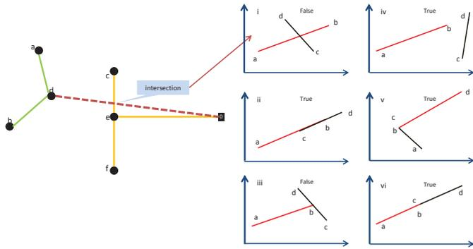
Solution(1/4): Add new line segments such that node crossings are detected by Non-crossing procedure
