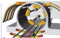
Based on adaptation of pipe-jacking techniques. Instead of using hydraulic jacks to push prefabricated concrete segments into a reception lane, a circular arrangement of jacks will 'launch' previously filled molds into a reception lane. A new set of forms are then interlocked with the previous, filled with fresh concrete and launched again. All concreting operations are located at a fixed location
