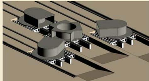
Prior to cast prestressing ducts in the existing pieces will also be properly connected and prepared for the post-tensioning process. The cables will be tensioned and grouted when the concrete in the pontoon joints has reached sufficient compressive strength, typically 1-2 weeks after casting. The tendons in the base slab will be tensioned when pontoon walls are cast. The top slab tendons will be tensioned after slip forming of the first part of the central shaft and corner columns.
