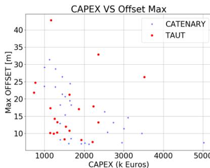
Figure 3 : CAPEX versus station keeping performance
