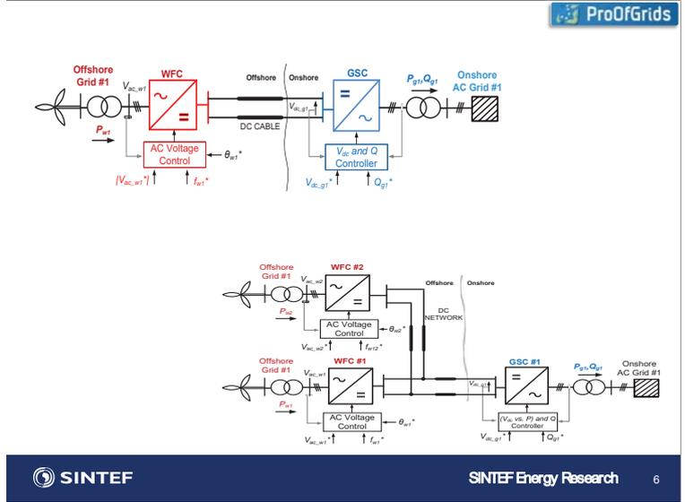
The top diagram shows a single WFC (Voltage Fed Converter) connected to an AC grid via a DC cable. It includes an AC Voltage Control block and a GSC (Grid Side Converter) block. The bottom diagram shows a more complex configuration with two WFCs and a GSC connected to an AC grid via a DC network.
