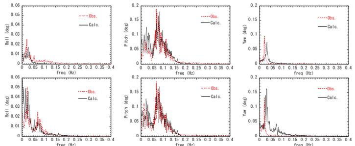
Figure. Amplitude spectra of the floater rotational motion for the aligned case (Upper Row) and the misaligned case (Lower Row)
