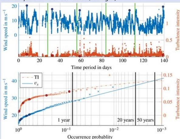
Fig. 1: Top: Wind speed and TI data of 24 weeks. 4 week periods and selected peaks are marked
