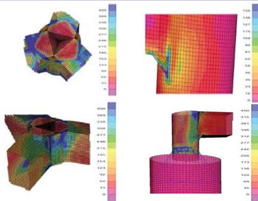
Critical points of tri-spar floater considered for ULS and FLS verification. Stress contours from ULS case II (max moment at gamma connection).
