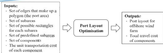
Optimal layout of the port given the dimensions and travel costs
