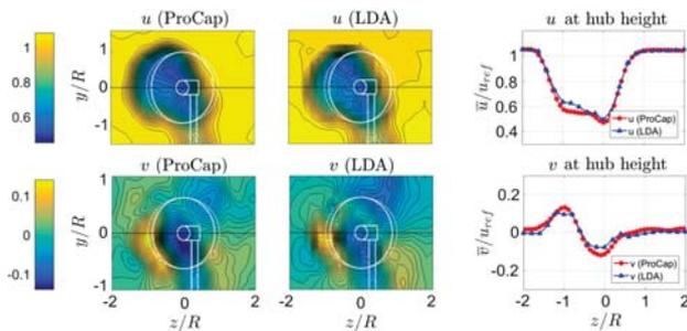
Comparison of the measured flow component  $u$  and  $v$  at  $x/D = 3$  and  $\gamma = 30^\circ$ .
