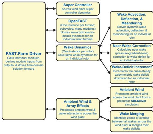
The diagram shows the FAST.Farm Driver at the center, which calls individual modules and drives time-domain solution forward. The modules are:
