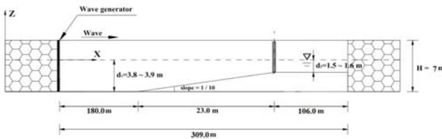
Fig 2. Experimental set up in GWK [3]
