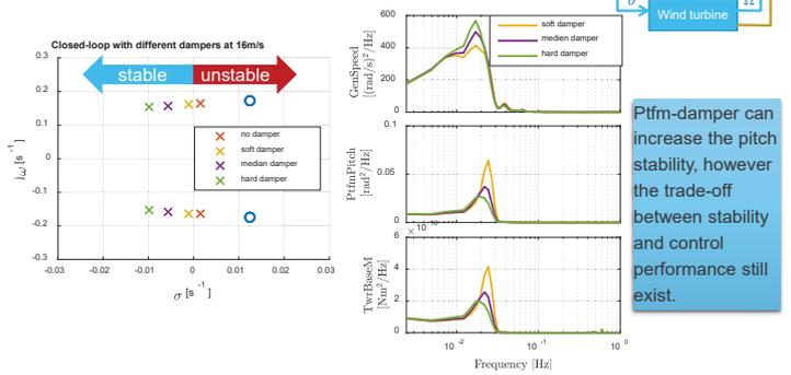
Ptfm-damper can increase the pitch stability, however the trade-off between stability and control performance still exist.
