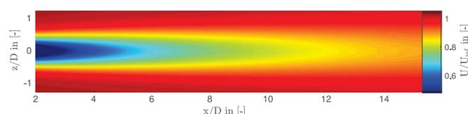
Figure 3: Adjusted Jensen-Gaussian Wake Model simulation result
