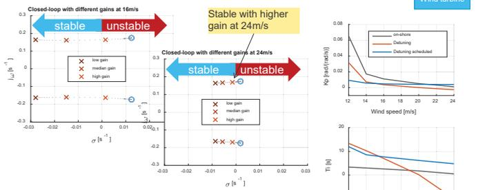
RHPZ problem differs from the operating wind speed, thus detuning should be applied according to the operating point
