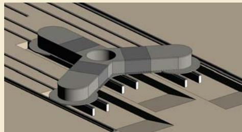
Estimated time for completing the star pontoon at Station 2, including enough curing time before skidding, is typically 1 month.
