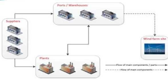
Optimal arrangement of supply chain (suppliers, manufacturers/plants, and warehouses (ports)) and schedule from the production of turbine parts to delivery at port.
