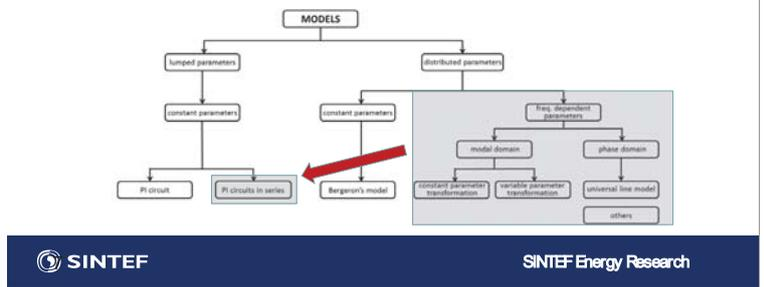
The diagram shows a hierarchy of models: Lumped parameters (PI circuit, PI circuits in series) and distributed parameters (Bergman's model, frequency-dependent elements in modal and phase domains, constant and variable parameter transformations, universal line model, and others).
