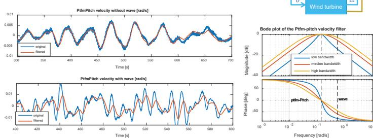
Due to the difficulty on filtering out the signal in wave frequencies, Ptfm Damper doesn't work well for Ptfms with pitch eigen-frequency close to the wave frequencies,
