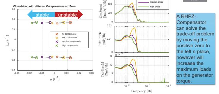
A RHPZ-Compensator can solve the trade-off problem by moving the positive zero to the left s-plane, however will increase the maximum loads on the generator torque.
