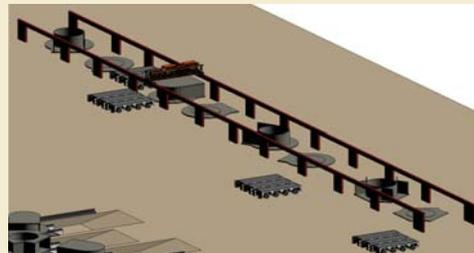
**Station 2:** The pontoon parts are accurately placed with a separation between the parts. The pre-fabricated pontoon parts will have protruding rebars, and splicing rebars will fill the gap between the parts. The concrete joint surface will be cleaned and prepared for proper bonding to the fresh concrete which will be cast in-situ to fill the gaps.
