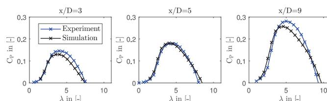
Figure 4: Downstream turbine power measurement and modelling comparison
