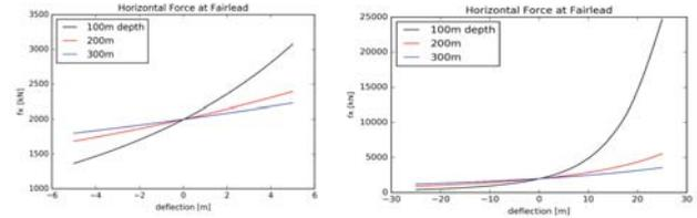
Decreasing water depth gives decreasing catenary effect and increasing force amplitudes for given floater motions
