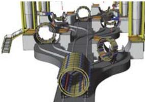
As long as  $t_{waiting} \ll t_{setting}$  concrete joints between rings will not form. To ensure bonding, extra concrete can be pumped radially at the interphase of a completed ring while waiting for the next ring to be connected. Train-like bogies and rail tracks allow swift transport of freshly filled molds.
