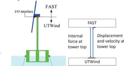
Figure. Outline of the coupling of NK-UTWind and FAST
