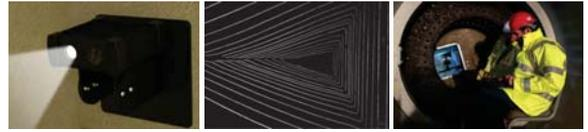
BOHEM's robust root mounted vision system tracks the displacement of a series of reflective markers installed in the blade's most critical areas. The reflective markers are passive, low cost, easy to install and can be removed without damage to the blade.
