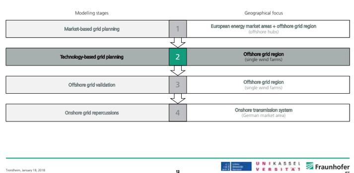
Technology-based grid planning stage simultaneously optimises locations of future wind farms, their connection(s) to shore, and the main technical components
