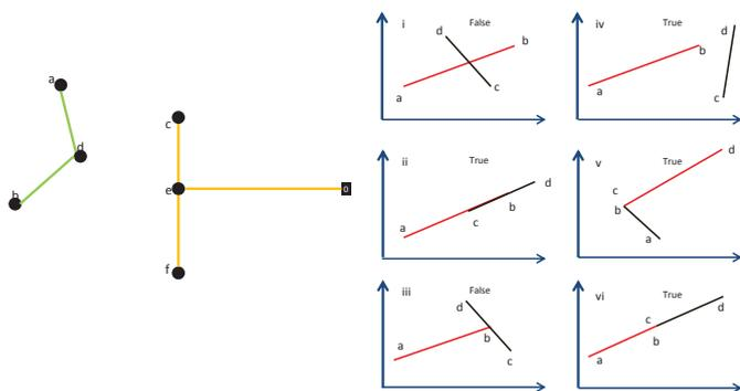
Solution(3/4): Add new line segments such that node crossings are detected by Non-crossing procedure
