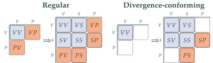
The system matrix (size  $2N$ ) will usually have a rank-deficient velocity-pressure block (VP, indicated with dashed lines). Enriching the velocity space with so-called *supremizers* ensures a full-rank system matrix with size  $3N$ . A divergence-conforming method will produce a fully divergence-free basis, so the VP-block vanishes, giving a block-triangular system, solvable as two size- $N$  systems instead of one size- $3N$  system.
