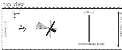
Full plane, Laser Doppler Anemometer measurements
