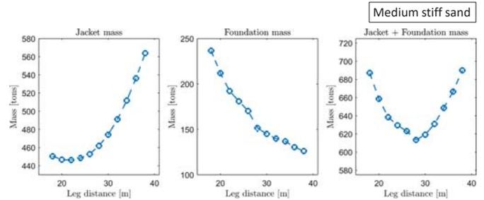
For a given design problem (10 MW turbine, 50 m depth, piles), the total mass was minimized to 631 tons (in 5 minutes on a laptop)
