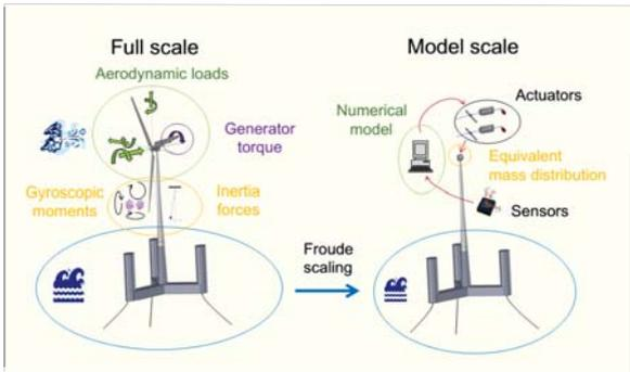
ReaTHM® testing circumvents limitations of hydrodynamic laboratories, and in particular inherent issues of physical wind/wave testing of floating wind turbines. The rotor and wind field are numerical and interact in real time with the scale model subjected to physical hydrodynamic loads, by means of sensors and actuators.
