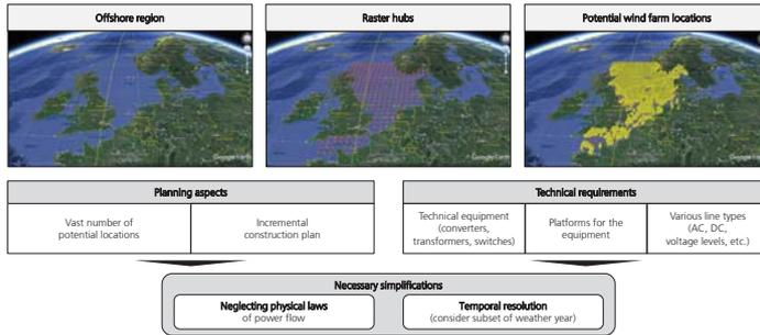
Due to a large number of time steps and scenarios, an automated approach was developed to electrically validate the market- and technology-based grid planning results
