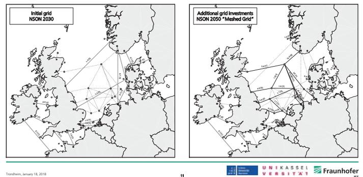
The large-scale offshore grid expansion planning model has a particular focus on capturing future energy system flexibility in the onshore market areas
