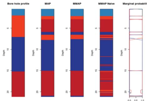
Figure 2: Training CPT profile, non-strict transition matrix: actual soil class profile, model predictions (MAP, MMAP and NB) and marginal probabilities.
