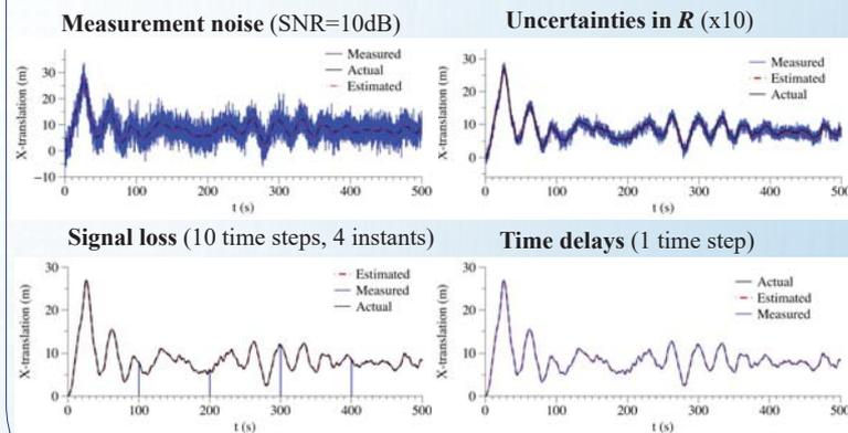
The estimator is robust towards noise, uncertainties, time delays and signal loss.
