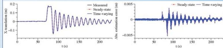
Comparison of steady-state and time-varying Kalman estimates with physical data
