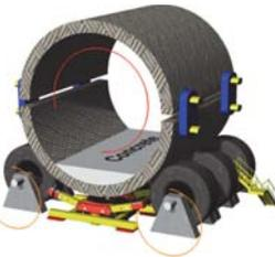
Compaction by centrifugation is a technique typically limited to  $\phi$  1-2m, arguably applicable to a  $\phi$  13 m of the tower. Plus, spinning the 200-m long structure, if at all possible, results in unprecedented up-scaling in terms of equipment and energy and presents unreasonable execution risk (many spinning devices perfectly synchronized). Centrifuging discrete segments is the only realistic option but results in a non-monolithic structure.
