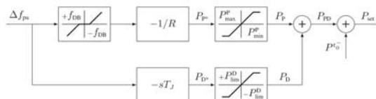
Fig. 8: Block diagram of the frequency support requirement
