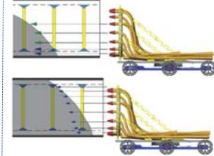
Pumping rate should be more intensive at the lower part to create a concrete slope within forms so concrete placed at higher levels has a base to fall on. Slope angle must be such that freshly pumped concrete does not slide off. Pumphines must be extendable and can rest on reinforcement bars not yet reached by concrete. New forms must be in place before the previous are completely filled whilst pouring never stops. The device slides backwards as construction progresses.
