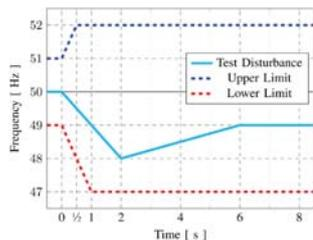
Fig. 6: Disturbance ride through requirement
