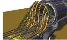
Comparable to slipforming in the sense that concrete is introduced axially, perpendicular to the cross-section of the tower into previously erected forms. The fundamental difference is how concrete is placed, linked to the fact that the device moves horizontally instead of vertically.
