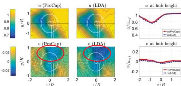
Comparison of the measured flow component  $u$  and  $v$  at  $x/D = 6$  and  $\gamma = 30^\circ$ .
