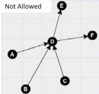
The out-degree of each turbine node must be one. However, in-degree can be more which is referred to as **branching**.
