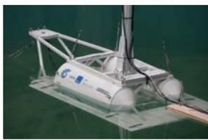
Fig 2. Scale model of SATH, in the CCOB in IHCantabria, right before a wave test.
