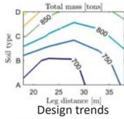
Structural optimization is used to automate the "well-defined" engineering tasks of conceptual support structure design
