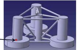
Pressure checking point: inner wall of upper column at lowest position
