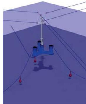
Figure 2: The OO-Star Wind Floater modelled in SIMA
