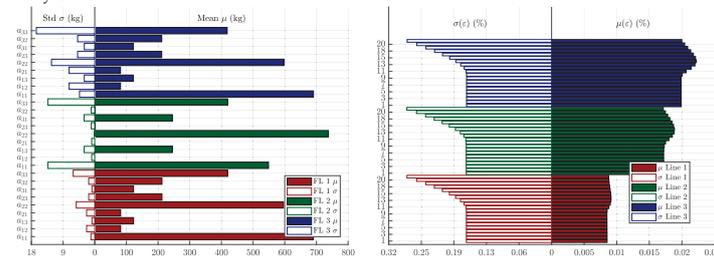
Figure 3: Added mass  $[a_i]$  contribution (Eq.6) for the node #20 for the combined decay tests  $\underline{x} = \{x, y, z, \varphi, \theta, \psi\}^T = \{20\text{ m}, 20\text{ m}, 10\text{ m}, 15^\circ, 15^\circ, 15^\circ\}^T$  (left) and strain  $\epsilon$  contribution for the internal nodes (#2-20) in the same decay tests (right).
