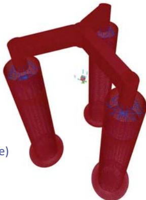
INNWIND 10MW tri-spar concrete floater
