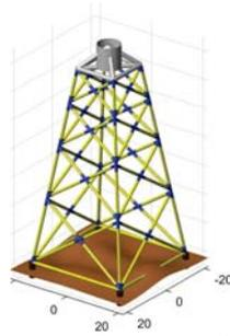
When support structures with different leg distance are optimized, jacket mass and foundation mass show opposite design trends
