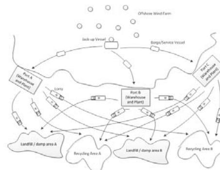
Vessel schedule and flow of components for decommissioning. The objective function is to minimise the total cost of activities.
