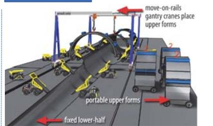
The giant re-usable mold, in which the bottom half is fixed and spans the entire length of the structure while the top half are a series of removable arch-forms. This method allows simultaneous pouring of the whole structure with directly discharging dumpster trucks and other high-throughput placement systems.
