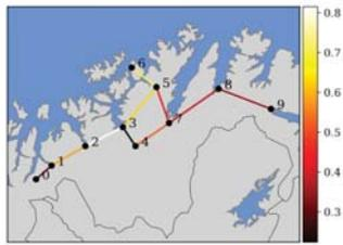
Figure 2: Case study system based on the power system in Finnmark, northern Norway. Lines are colored according to the line utilization in the run with 120 wind power samples. Power is on average flowing from both ends towards node 6.
