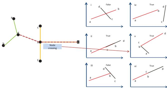
Solution(2/4): Add new line segments such that node crossings are detected by Non-crossing procedure
