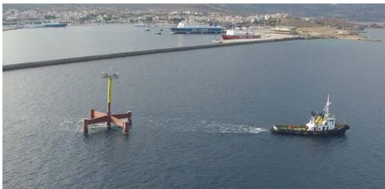
FloatMast TLP Platform tugging at Test Site
