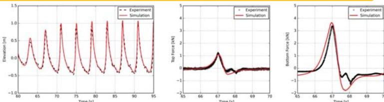
Fig 6. Wave surface elevations simulated in OceanWave3D agree well with experimental data. Response force for a non-breaking wave are simulated in HAWC2 with the wave kinematics from OceanWave3D showing good agreement with measurements
