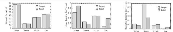
Figure. Comparison of calculated and measured natural period (left), linear damping coefficient (middle) and quadratic damping coefficient (right)
