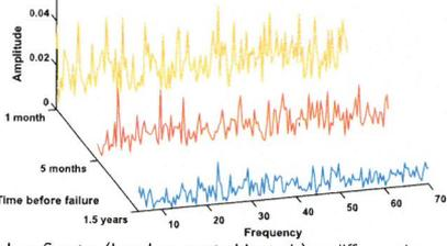
Figure: Envelope Spectra (based on spectral kurtosis) at different times prior to failure.
