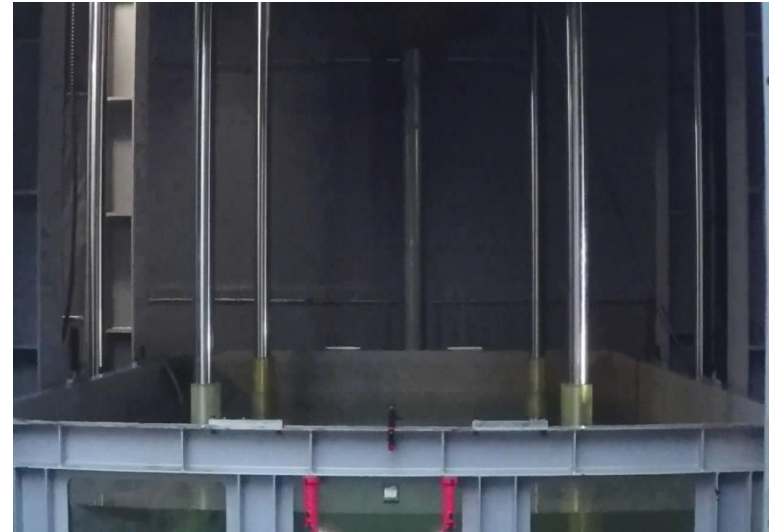
➤ Steel - Dead-rise angle 10°, Drop height : 1.7m
