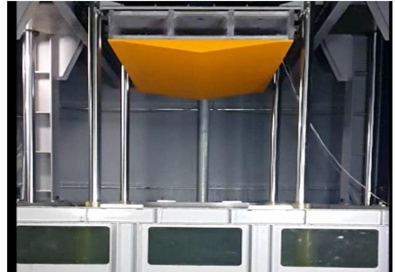
➤ Wood - Dead-rise angle 10°, Drop height : 1.7m
