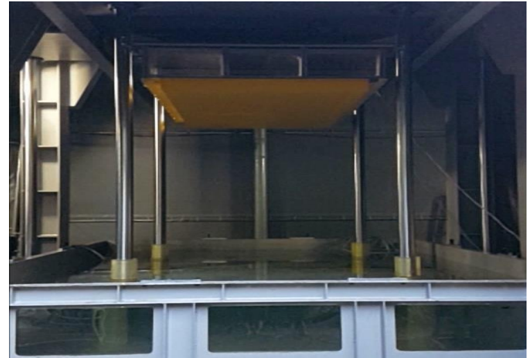
➤ Wood - Dead-rise angle 0°, Drop height : 1.7m
