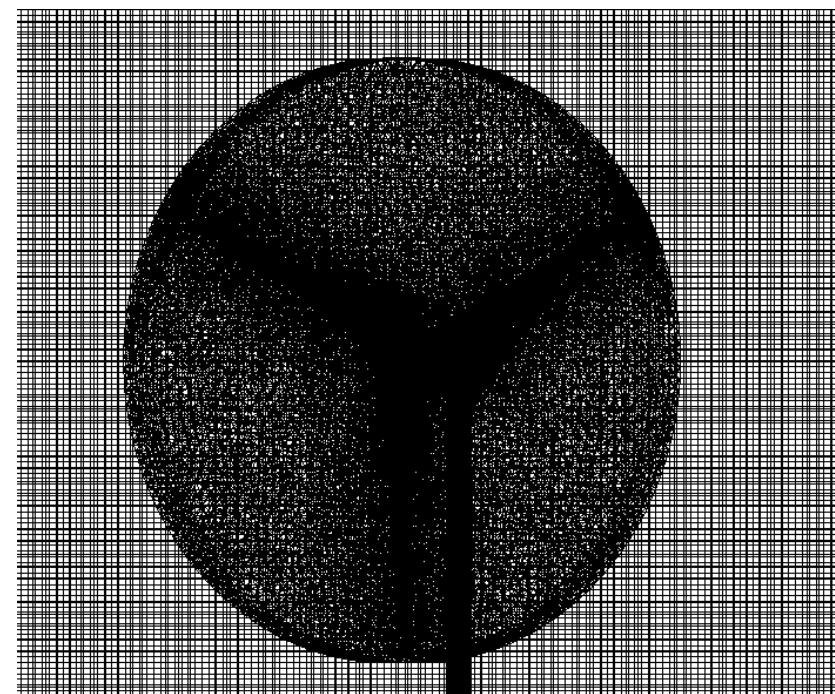
(b) Sliding mesh and grid size
