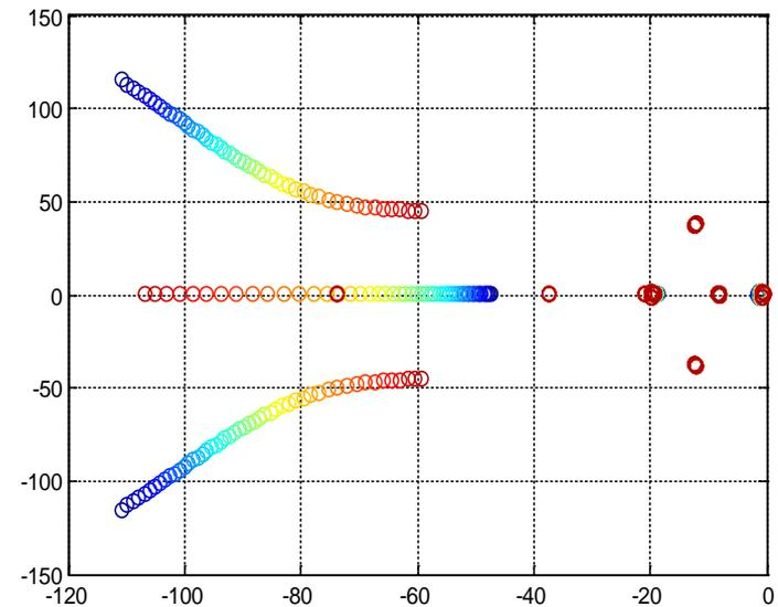
Trajectory of critical eigenvalue with power reference is varied from -1.0 to 1.0 pu
