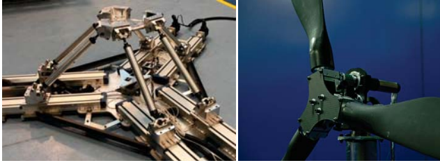
Figure 2: HexaFloat robot [5] (left) and fully controlled 1/75 aero-elastic scale model of the 10 MW DTU reference wind turbine (right), [6], [7].
