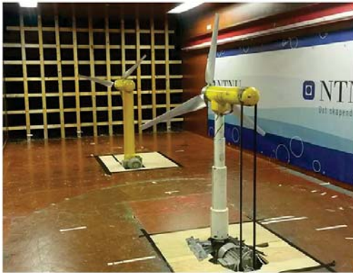
Figure 1: Two aligned turbines in the NTNU wind tunnel
