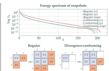
The system matrix (size 2N) will usually have a rank-deficient velocity-pressure block (VP, indicated with dashed lines). Enriching the velocity space with so-called *supremizers* ensures a full-rank system matrix with size 3N. A divergence-conforming method will produce a fully divergence-free basis, so the VP-block vanishes, giving a block-triangular system, solvable as two size-N systems instead of one size-3N system.
