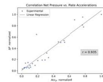
Fig 8. Correlation graph for the normalized pressure and plate's normal acceleration.
