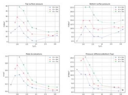
Fig 7. Pressure magnitude and plate accelerations for 3 different wave heights and by incident wave to natural heave period.
