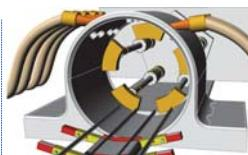
Based on adaptation of pipe-jacking techniques. Instead of using hydraulic jacks to push prefab concrete segments into the soil, a circular arrangement of jacks will "launch" previously filled molds into a reception lane. A new set of forms are then interlocked with the previous, filled with fresh concrete and launched again. All concreting operations are located at a fixed location.
