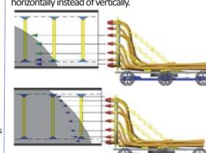
Pumping rate should be more intensive at the lower part to create a concrete slope within forms so concrete placed at higher levels has a base to fall on. Slope angle must be such that freshly pumped concrete does not slide off. Pump lines must be extendable and can rest on reinforcement bars not yet reached by concrete. New forms must be in place before the previous are completely filled whilst pouring never stops. The device slides backwards as construction progresses.
