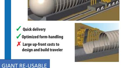
Tolerating a certain number of joints may result in a cheaper construction process. The cost reduction in construction by allowing joints in a segment approach will need to be compared to the costs of high-quality sealing of these joints, the increased maintenance costs and the impact on the life-time of the structure.
