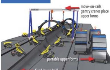
The giant re-usable mold, in which the bottom half is fixed and spans the entire length of the structure while the top half are a series of removable arch-forms. This method allows simultaneous pouring of the whole structure with directly discharging dumpster trucks and other high-throughput placement systems.
