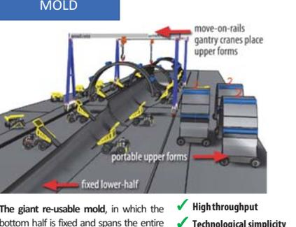
As long as  $t_{waiting} \ll t_{setting}$  concrete joints between rings will not form. To ensure bonding, extra concrete can be pumped radially at the interphase of a completed ring while waiting for the next ring to be connected. Train-like bogies and rail tracks allow swift transport of freshly filled molds.
