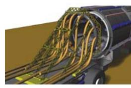
Comparable to slipforming in the sense that concrete is introduced axially, perpendicular to the cross-section of the tower into previously erected forms. The fundamental difference is how concrete is placed, linked to the fact that the device moves horizontally instead of vertically.
