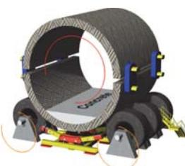
Several identical "casting stations" operate in staggered cycles with a fixed lag time  $t_{lag}$  (e.g. 15 min between the start of two consecutive stations) and produce identical rings. It takes each station a time  $t_{production}$  to complete a ring. Once a given ring has been completed its transported to the assembly line where it "waits" in place during  $t_{waiting} = t_{lag}$  before the next ring produced at the consecutive station is ready to be connected.
