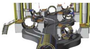
As long as  $t_{waiting} \ll t_{setting \text{ concrete}}$  joints between rings will not form. To ensure bonding, extra concrete can be pumped radially at the interface of a completed ring while waiting for the next ring to be connected. Train-like bogies and rail tracks allow swift transport of freshly filled molds.
