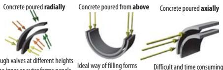
Through valves at different heights on the inner or outer forms panels
