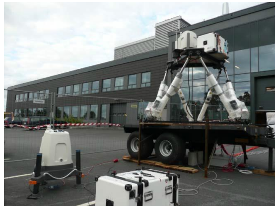
Photo 2: CMR's experimental setup [8] for motion induced errors in wind speed: Two fixed lidars against two identical ones on a moving platform.
