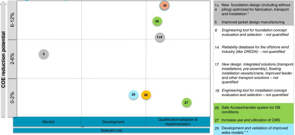
\*Reduction potential number from Offshore Wind Accelerator for concepts at 35 m water depth
