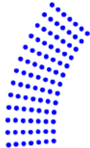
Horns Rev 2 (HR2) 91x2.3 MW Hub height: 68 m Rotor diameter: 93 m
