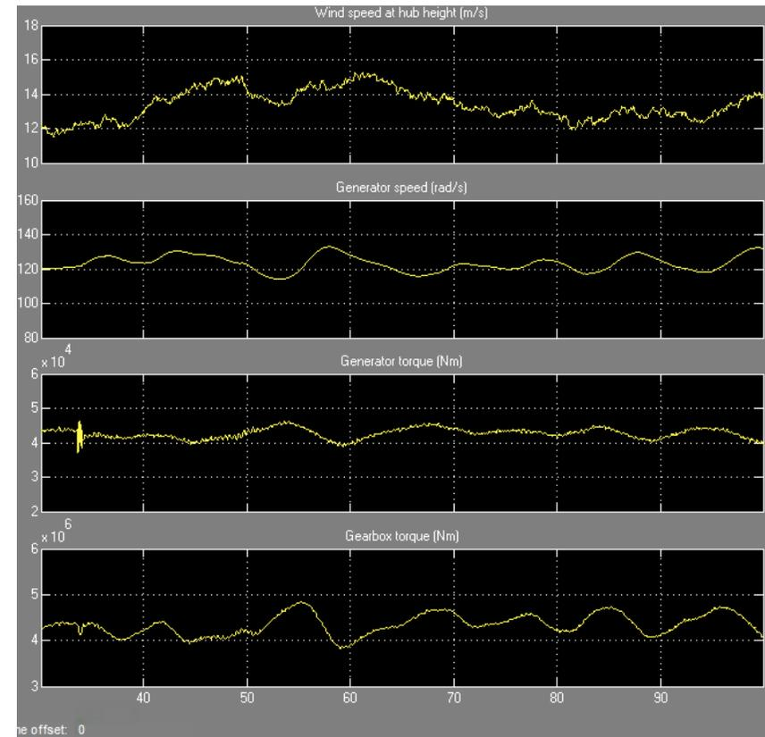
Responses without and with gearbox vibration control loop mitigation
