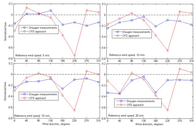
Fig. 2. Normalized bias of the wind speed measured at the platform and obtained during the CFD analysis plotted for different wind directions
