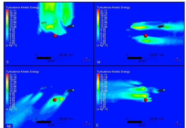
Fig. 3. Turbulent kinetic energy contours plotted on a cross-section plane for 4 cases with 15 m/s wind speed and different wind directions
