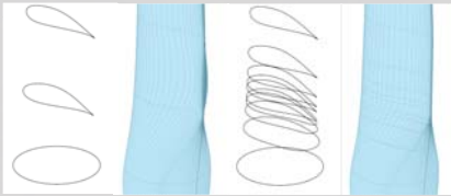
Figure 1: 3D turbine blade geometry may be generated by lofting the given cross-sections
