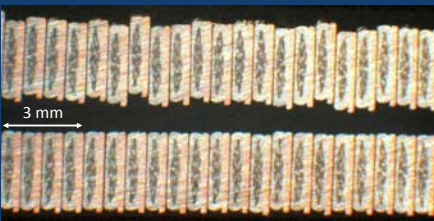
Cross-section of first double pancake winding trial
