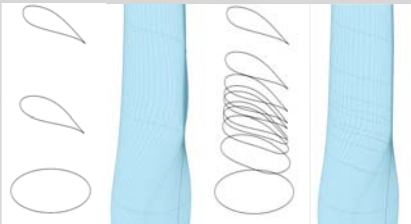
Figure 2: Two-step interpolation routine with low and high order avoids a self-intersecting mesh.
