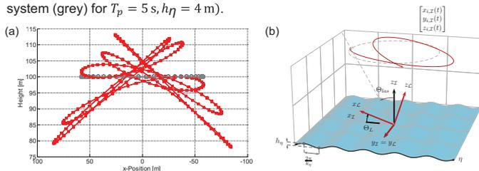
Fig. 1: (a) Lidar measurement points for  $t = 20$  s, (b) one single measurement trajectory  $t = 1$  s, for a fixed (grey) and moving (red) lidar with focus length  $f = 100$  m.
