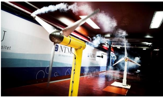
Fig. 1: Blind test 2 setup of two model wind turbines in NTNU's wind tunnel
