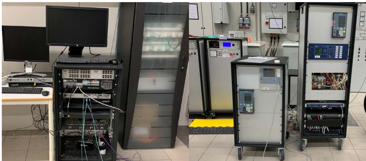
Figure 11 NSGL flexible digital substation equipment. (Left) DRTS from OPAL-RT and optic fibre rack. (Right) Multiple vendor MUs, IEDs, GPS clock and communication switches.
