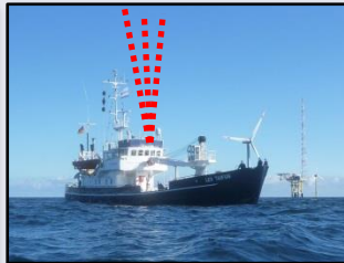
Figure 2: Ship-lidar measurement in proximity to offshore meteorological mast FINO1. Position of the lidar system is indicated by the red beam lines.
