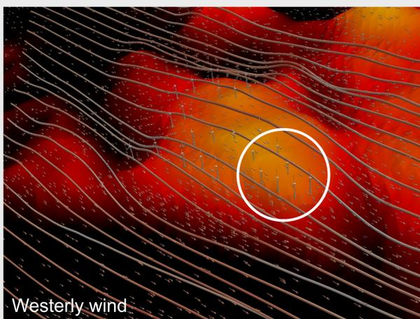
Stream lines for two most dominant wind directions. The figure clearly shows that the wind has a tendency to go around the hill which is perhaps related to the strong stratification in the region thus avoiding a few turbines which consistently underperform.
