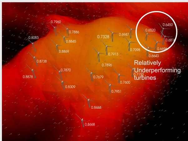
Offline simulations conducted with the most frequently encountered wind and stratification conditions:
