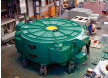
PM generator from Siemens. 3 MW, 17 rpm
