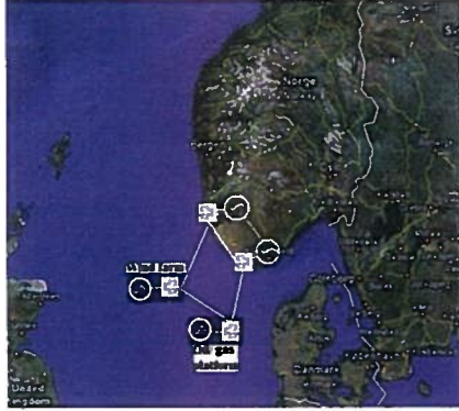
Figure 1: Early stage scenario of multiterminal HVDC in the North Sea
