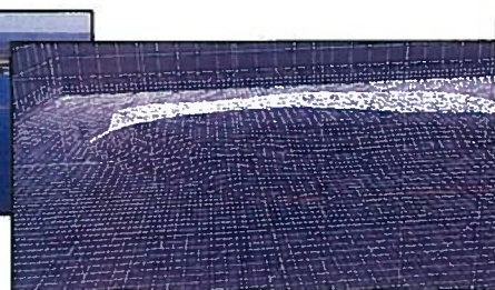
Bolund mesh created by the use of openFoam's snappyHexMesh
