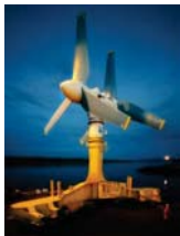
1.1 MW tidal turbine of Atlantis Resource Corporation (delivered)
