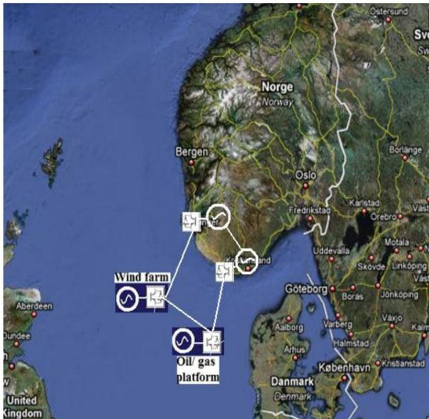
Figure 1: Early stage scenario of multiterminal HVDC in the North Sea
