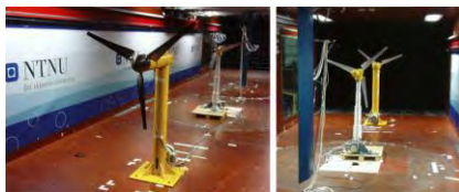
Figure 2: Tandem Setup in the wind tunnel.
