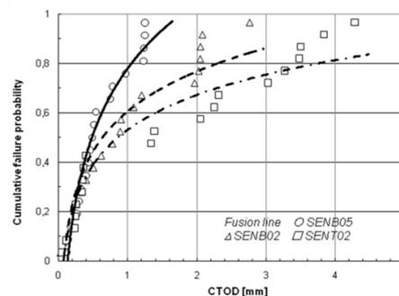
Figure 1. Large scatter in fusion line fracture toughness of 420 MPa steel.
