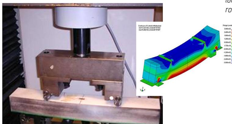
Fig.3. 4-point bending of pipeline insulation (left), and modelling of strain levels during 4-point bending (right).
