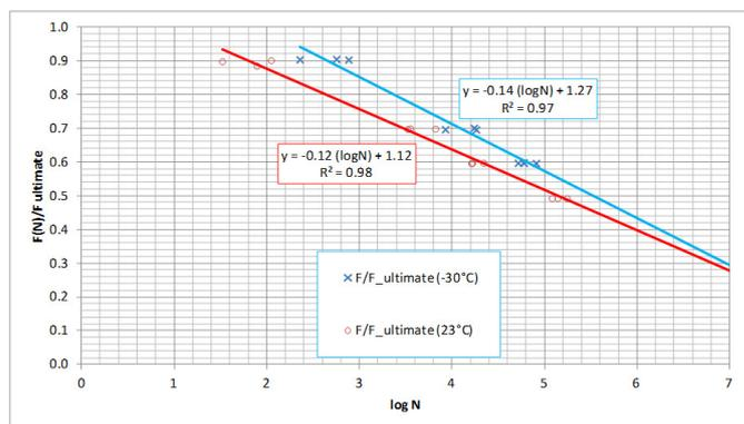
Figure 4. Results from low temperature fatigue testing of epoxy laminate with quadriaxial glass fibre reinforcement. Red curve – room temperature, blue curve – -30°C
