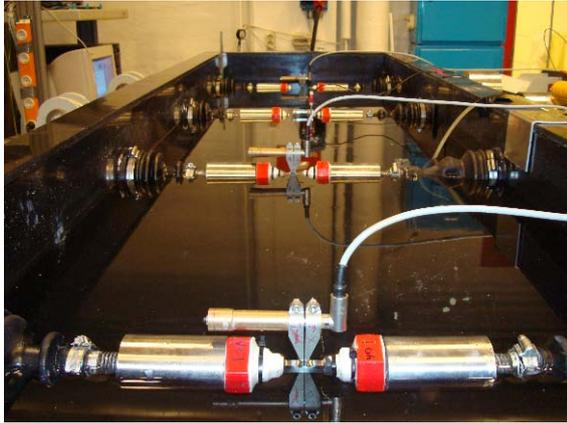
Figure 6 Test set up for the constant load SENT testing at CP conditions.
