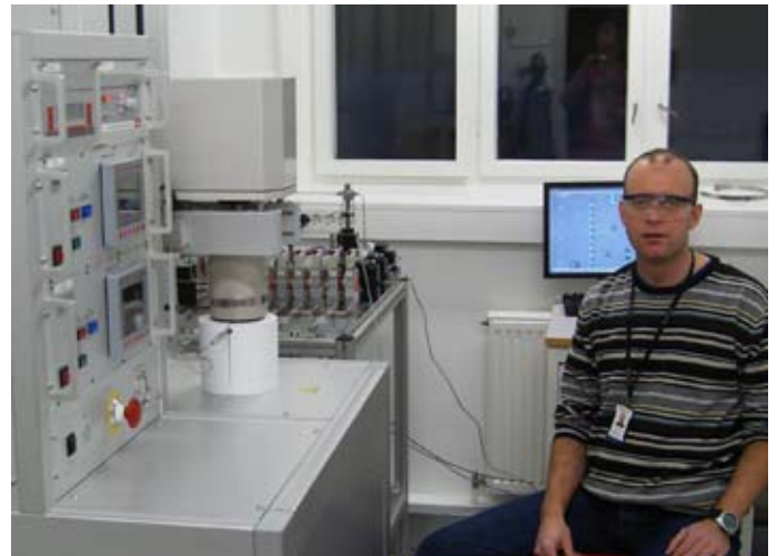
High-pressure magnetic suspension balance commissioned at SINTEF
