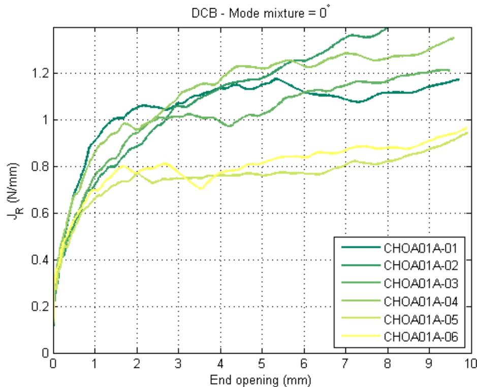
The A-series of DCB tests (0° mode mixture) showing high  $J_R$  values for specimens 01 and 04, and low  $J_R$  values for specimens 05 and 06
