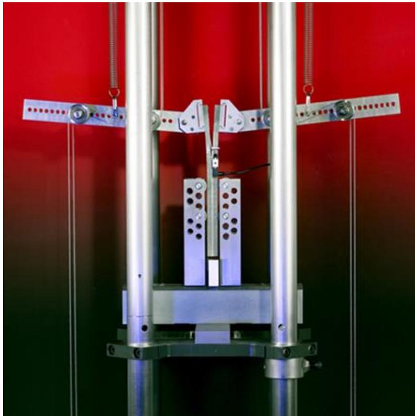
*Image showing a Dual Cantilever Beam (DCB) crack opening test where the resistance to crack growth can be measured*
