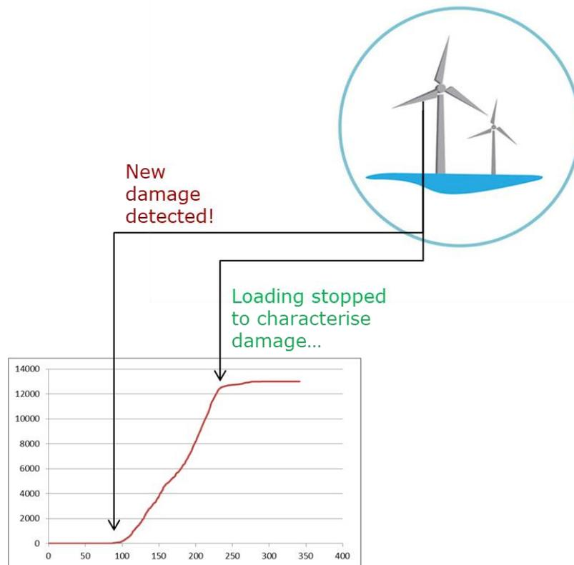
*Illustration of the Lvl 1 SHM monitoring concept warning that new damage has been detected within the structure*
