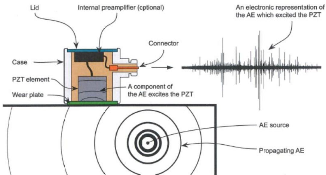
*Image from Unnþórsson (2013) showing the Acoustic Emission measurement principle*
