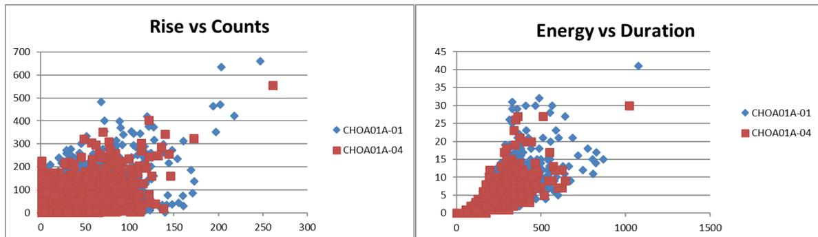
Scatter graphs showing (Rise time vs ring-down Counts) and (Energy vs Duration) for the AE hits detected in the A-series 01 and 04 specimens only
