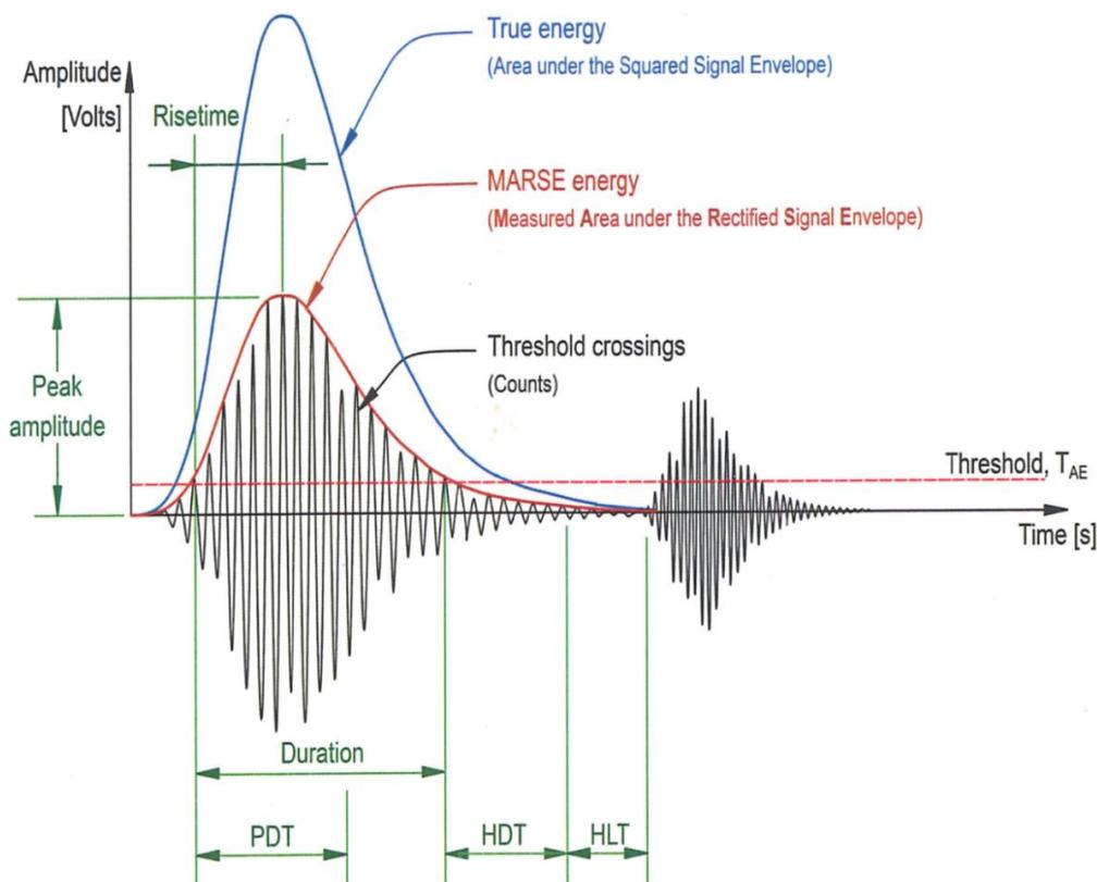
Image from Unnþórsson (2013) showing the Acoustic Emission waveform characteristics
