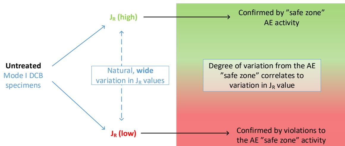
*Illustration of the “natural, wide” distribution of  $J_R$  values that can be confirmed in laboratory testing using AE measurements*
