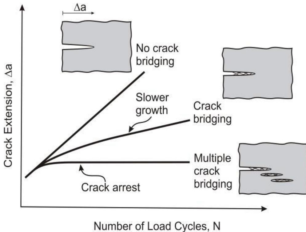
*Sketch from the DACOMAT project application (NMBP-06-2017) showing the effect of crack bridging and multiple cracks on crack extension as a result of the number of load cycles*
