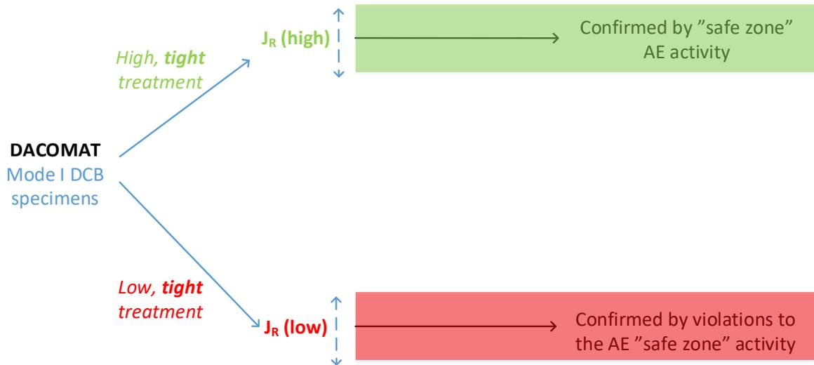
Illustration of the DACOMAT interface modifications to achieve a "high, tight" or "low, tight" distribution of  $J_R$  values, and confirmation of the effect via the laboratory test AE measurements
