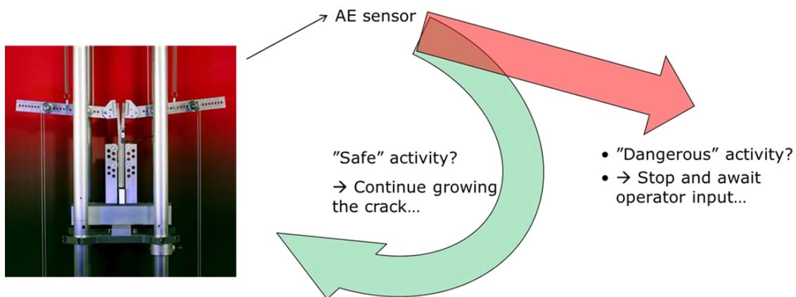
Illustration of an automated damage control mechanical test
