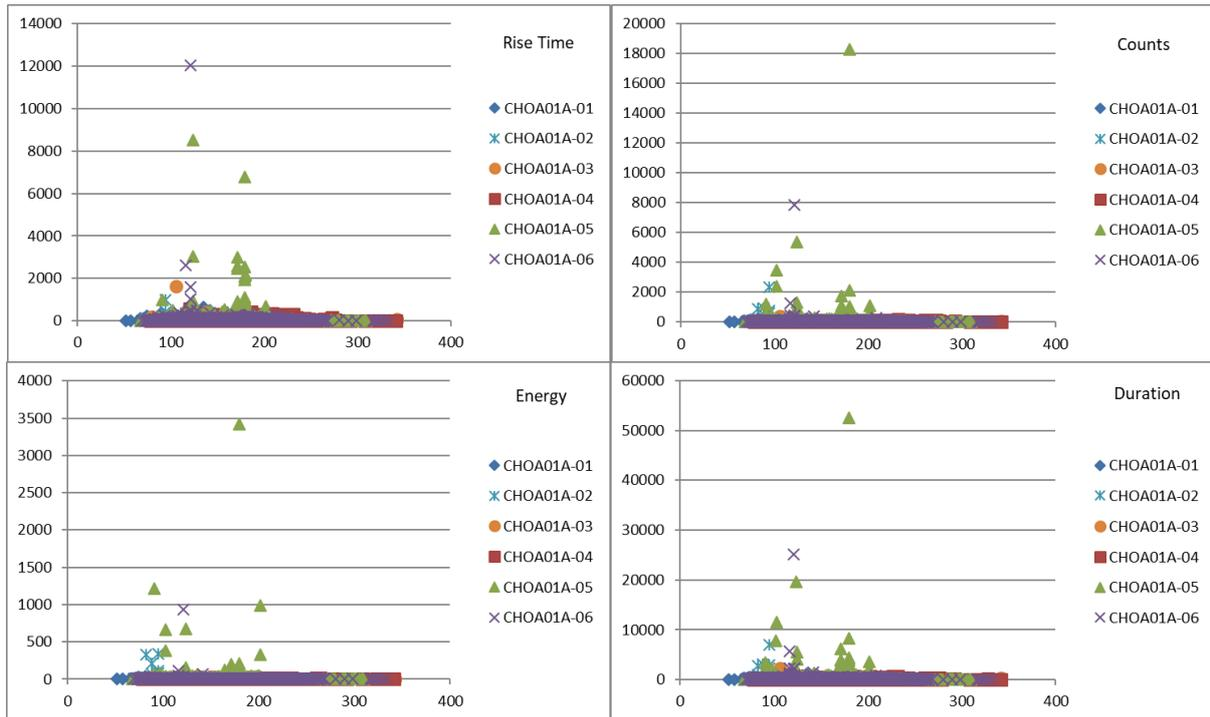
Graphs showing the distribution of values for the AE measurements on all six A-series specimens
