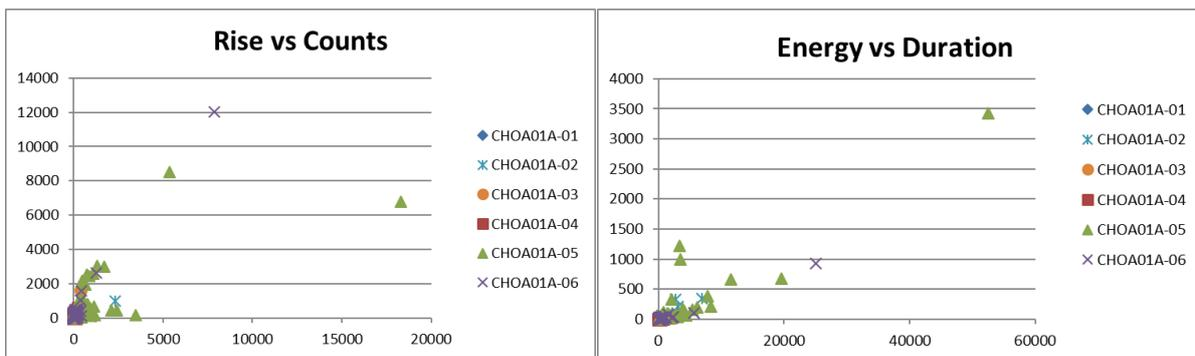
Scatter graphs showing (Rise time vs ring-down Counts) and (Energy vs Duration) for the AE hits detected in all six A-series test specimens
