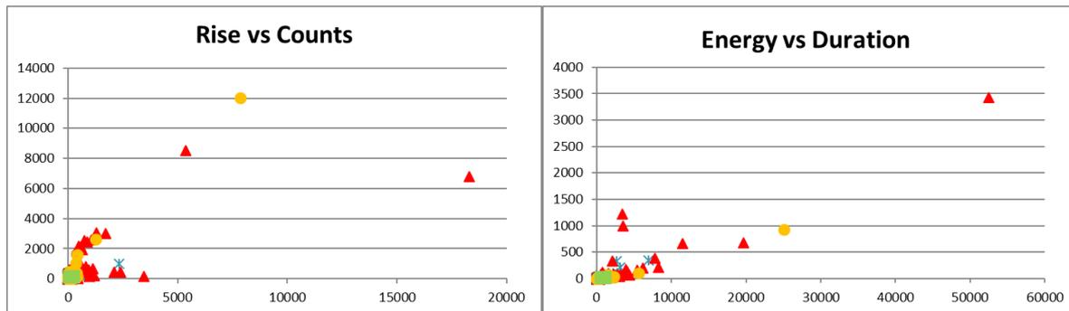
The Series-A scatter graphs showing the green square “safe zone” where all AE activity from the high  $J_R$  test specimens is contained. Only specimens with low  $J_R$  generate any AE outside this zone.
