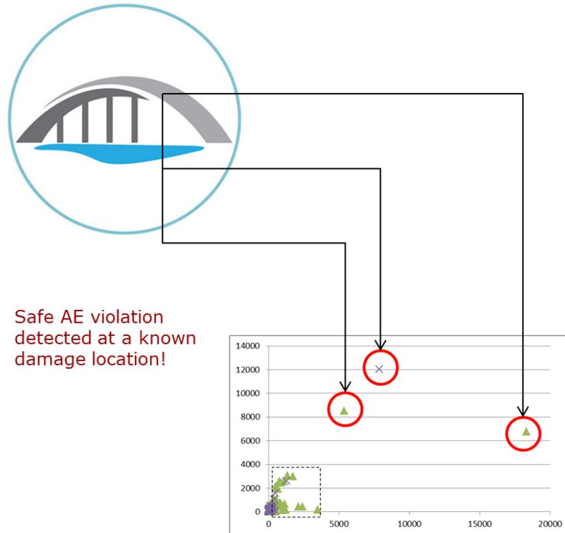
*Illustration of the Lvl 2 SHM monitoring concept warning that a known damage area is violating the DACOMAT “safe zone” for AE activity and possibly no longer providing the desired damage tolerance*
