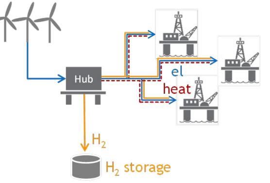
Provide clean heat and electric power to clusters of offshore oil&gas production facilities and other potential future customers
