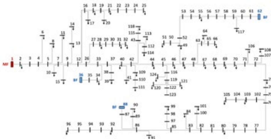
Figure 1 The CINELDI MV reference grid
