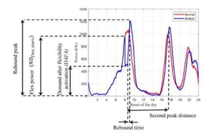
Illustration of the rebound effect of a water heater.
