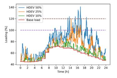
Transformer loading in a Norwegian transit area with increasing share of heavy-duty electric vehicles
