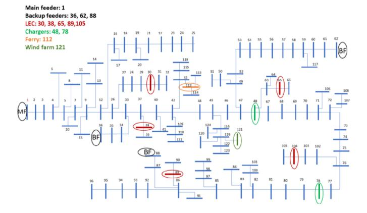
Figure 1. CINELDI 124 bus MV distribution reference grid for flexibility studies.
