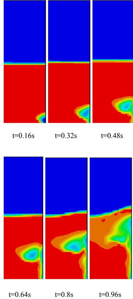
**Fig.2 Contours of solid volume fraction in the bed.**
