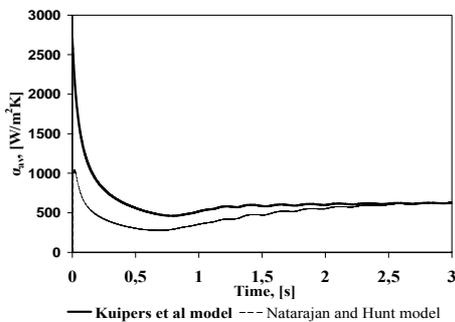
**Fig. 4b** Comparison between two solid phase thermal conductivity models.
