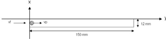
Figure 2: Sketch of the simple pipe.
