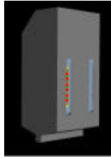
Figure 1: Schematic of the tangentially-fired boiler (with one burner assembly highlighted in multi-colours).
